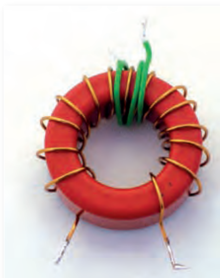
Close-up look at the inductor wound on a T130-2 toroid.
